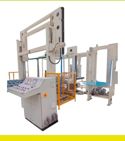
The block processing line machine is designed for complete processing of short & long foam blocks with a belt conveyor.
